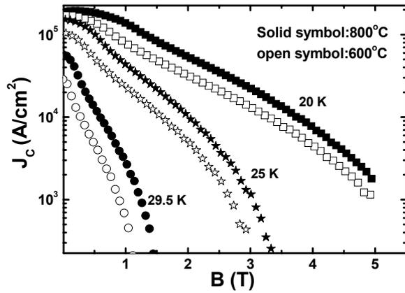
**Figure 1.** Magnetic and temperature dependences of the critical current density  $J_c$  for 600 and 800 °C reaction temperatures.
