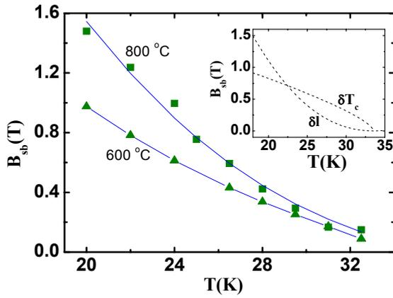
**Figure 3.** Temperature dependence of the crossover field  $B_{sb}$ . The solid curves are fits to eq. (3). Inset: The  $\delta T_c$  and  $\delta l$  pinning correspond to eq. (2).
