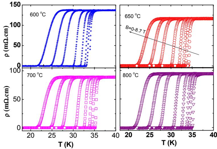
**Figure 6.** The electrical resistivity as a function of temperature in fields of 0-8.7 T for 10wt% malic acid doped  $\text{MgB}_2$  sintered at 600, 650, 700, and 800 °C.
