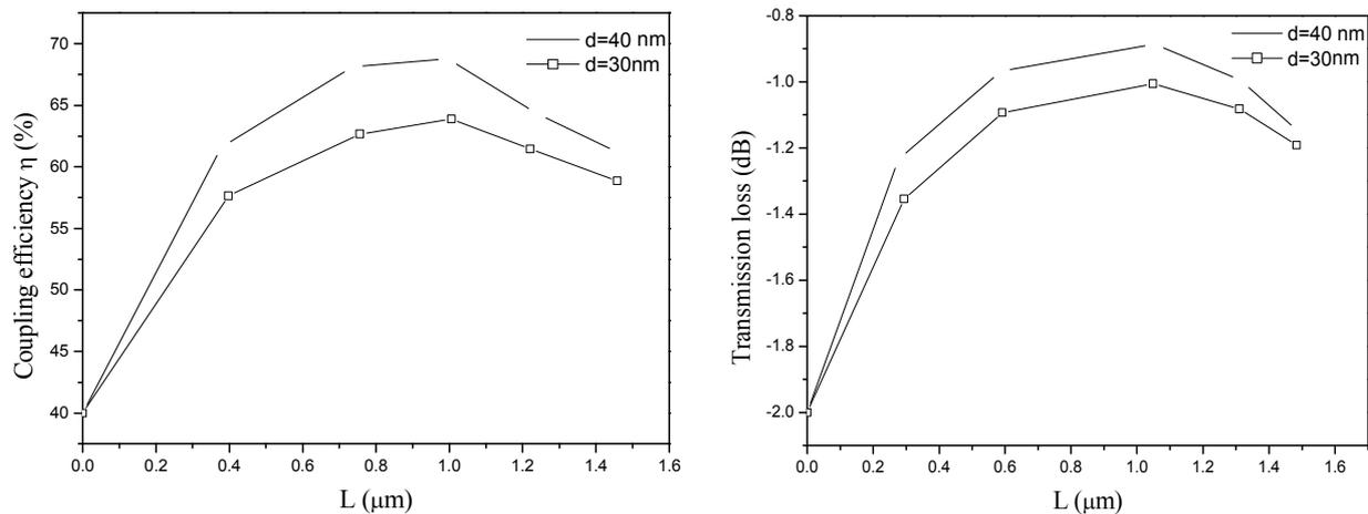
**Figure 2.** (a) Coupling efficiency (b) Transmission loss as a function of taper length when  $\alpha$  is set as  $60^\circ$  and  $l=300$ nm for two slot thickness values of  $d=30$  nm and  $d=40$  nm.
