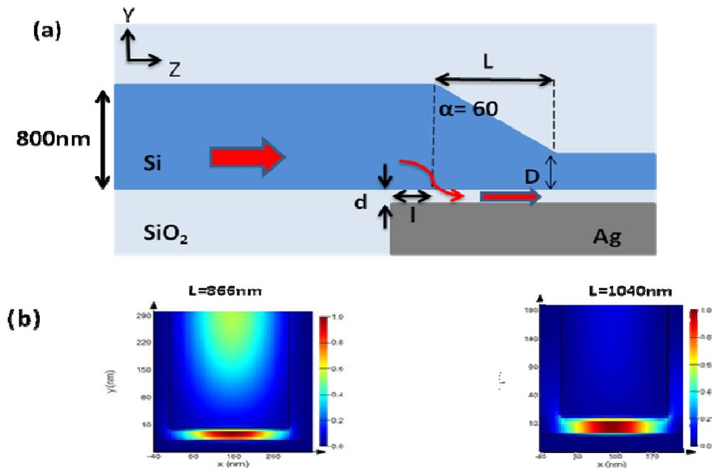
**Figure 1.** (a) Schematic diagram for the dielectric to hybrid plasmonic waveguide. (b) The electric-field distribution in the cross section XY-plane at two cross sections of  $L=1040$  nm and  $866$  nm when  $\alpha$  is set as  $60^\circ$  and  $d=40$  nm and  $l=300$  nm when  $\lambda=1550$  nm.
