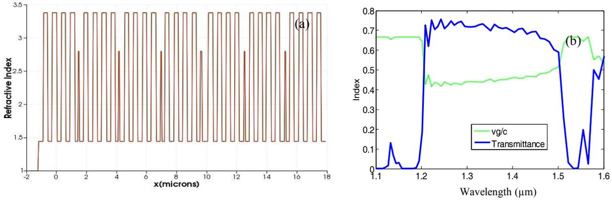
**Figure 1.** (a) Schematic illustration of the structure when the defect refractive index is  $n_{\text{defect}}=2.8$ . (b) Calculated transmission spectra and group velocity of the structure when  $n_{\text{defect}}=1.5$ .
