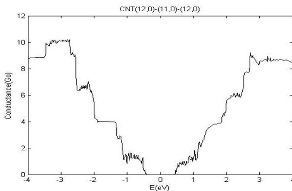
**Figure 3.** Conductance of the carbon nanotube (12,0)-(11,0)-(12,0).
