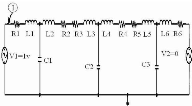
**Figure 4.** Circuit diagram for carbon nanotube metal-semiconductor-metal.
