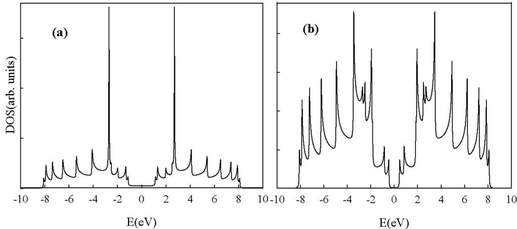
**Figure 2.** Densities of states in the isolated (12,0)-metallic and (11,0)-semiconducting nanotubes are illustrated in the right and left parts of the figure, respectively. All these curves are obtained from the recursion method. Small imaginary part is  $\eta = 0.02$  eV.
