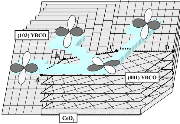
**Figure 1.** (color online) Sketch of the grain boundary structure in the bieftaxial technique.
