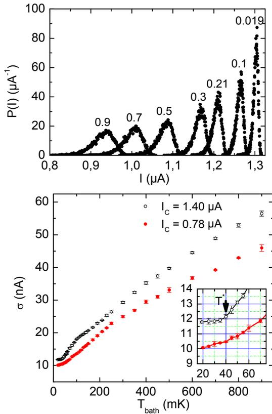
**Figure 3.** (color online) (a) Switching current probability distribution for different bath temperatures  $T_{\text{bath}}$ . The symbols represent data, and the lines are fits. (b) Temperature dependence of width  $\sigma$  for  $I_{c0}=1.40 \mu\text{A}$  and  $B=0 \text{ T}$  (open points) and  $I_{c0}=0.78 \mu\text{A}$  and  $B=2 \text{ mT}$  (full points). In the inset the low temperature part. (below 75 mK) is in evidence. Adapted from [11].
