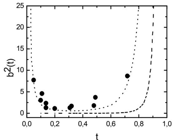
**Figure 5.** The behaviour of  $b^2$  vs the reduced temperature  $t = T/T_c$ . The dotted line represents the theoretical behaviour for the  $d$ -wave case, the solid line for the  $s$ -wave one-band case; the experimental points represent the results for standard high quality YBCO films at a circulating power of 0 dBm. Adapted from [49].
