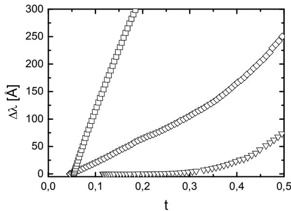
**Figure 4.** Low-temperature variation of the in-plane magnetic penetration depth for different superconductors: a Y124 single crystal ( $\square$ ), a Y123 single crystal ( $\diamond$ ), a NbN epitaxial thin film ( $\nabla$ ). Adapted from [50].
