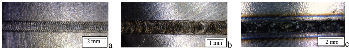
Figure 6. Surface appearance of A series: (a) A_1 (100% Ar), (b) A_4 (85% Ar + 15% \text{CO}_2 ), (c) A_6 (75% Ar + 25% \text{CO}_2 ).
