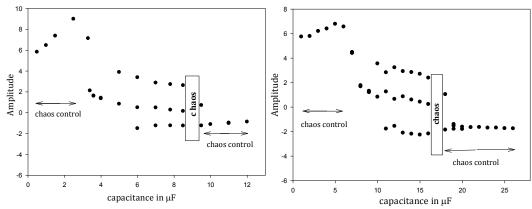
Figure 12. (left) Bifurcation diagram for the frequency f=400Hz and  $V_{in}=0.9$ V of the oscillator, showing chaos control regions and the highly chaotic region. (right) Bifurcation diagram for the frequency of 270Hz and  $V_{in}=0.9$ V of the oscillator, showing chaos controlled regions and the highly chaotic region.
