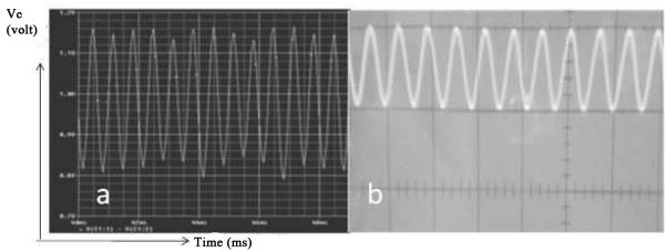
Figure 7. Time response of  $V_C$  giving the demise of chaos. Panel (a) PSPICE simulation. Panel (b) Experimental data.
