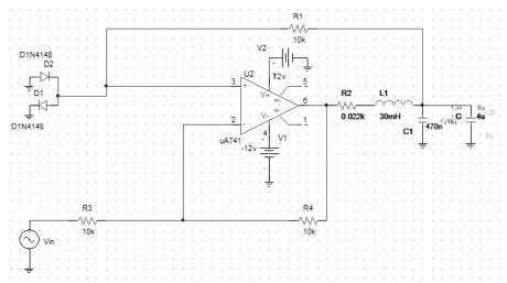
**Figure 10.** Circuit diagram for chaos control in the DH oscillator. Required change in capacitance is incorporated by putting C in parallel with C<sub>1</sub>.
