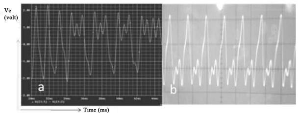
Figure 6. Chaotic time response of V<sub>C</sub>. Panel a: PSPICE simulation. Panel (b) Experimental data.
