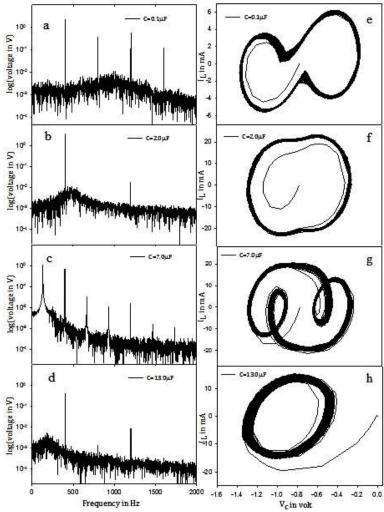
Figure 11. Power spectra and phase space diagrams varying the capacitance C (for  $V_{in}$ =0.9V, f=400Hz) of the oscillator. Left (a)-(d) panels are the spectra for C =0.1, 2.0, 7.0 and 13.0  $\mu$ F, respectively. Right panels (e-h) are the corresponding phase space ( $I_L$ - $V_C$ ) plots.
