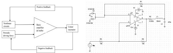
Figure 3. Left: The experimental electric circuit diagram. Right: The basic block diagram of the circuit.
