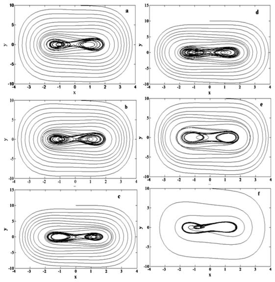
**Figure 2.** The MATLAB generated variation of the phase space plot with the frequency of the driving force. (a)  $\omega$ =0.193, b=0.9, a=0.087; (b)  $\omega$ =0.201, b=0.9, a=0.087; (c)  $\omega$ =0.231, b=0.9, a=0.087; (d)  $\omega$ =0.298, b=0.9, a=0.087; (e)  $\omega$ =0.440, b=0.9, a=0.087; (f)  $\omega$ =0.507, b=0.9, a=0.087. Symbols are used as described in the text.
