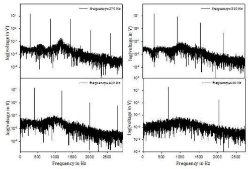
Figure 9. The input frequency driven power spectra of the DH oscillator circuit. f=270 Hz gives chaotic spectra. f=310Hz and 400 Hz show period 4 bifurcations, while f=680Hz is the period-2 only. The details are given in table 1.
