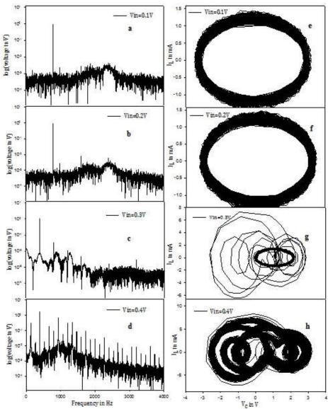
Figure 14. Power spectra and phase space diagrams for the synchronized oscillator circuit, as shown in Figure 14. Left (a)-(d) panels are the power spectra for the input voltage of the second oscillator, i.e  $V_{3c}$ =0.1, 0.2, 0.3 and 0.4 V, respectively. Right panels (e-h) are the corresponding phase space ( $I_L$ - $V_C$ ) plots.
