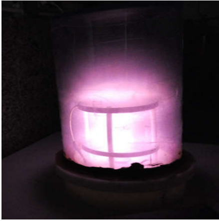
Figure 1. (color onlin) The photograph of plasma originated from Nitrogen by glow discharge between anode and cathode.
