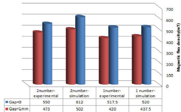
Figure 15. (color onlin) Measured and simulated values of one and two magnets in the surface and in a 1 mm distance from the surface.
