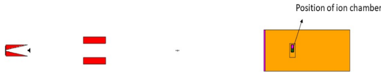
Figure 1. 2-D simulation geometry of linac including water phantom.
