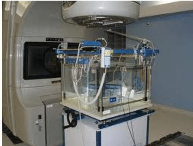
Figure 3. Experimental set-up for measuring TPR_{20,10} .
