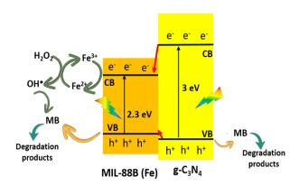
**Scheme 1.** Proposed mechanism of electron-hole generation, and transfer at the interface of g-C<sub>3</sub>N<sub>4</sub> and MIL-88B(Fe) under UV-Vis. light illumination, and the following photo-Fenton reactions at the surface of g-C<sub>3</sub>N<sub>4</sub>/MIL-88B(Fe) nanocomposite to degrade MB pollutant. (CB<sub>MIL-88B(Fe)</sub>=-1.55 eV, VB<sub>MIL-</sub> 88B(Fe)=0.73 eV, CB<sub>g-C3N4</sub>=-2.2 eV, VB<sub>g-C3N4</sub>=0.8 eV)
