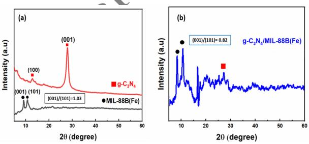
**Figure 3.** XRD pattern, (a) g-C<sub>3</sub>N<sub>4</sub> nanosheets, Metal-Organic framework MIL-88B(Fe), and (b) g-C<sub>3</sub>N<sub>4</sub>/MIL- 88B(Fe) nanocomposite.
