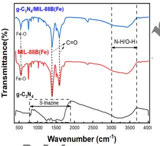
Figure 2. FTIR spectrum of g-C<sub>3</sub>N<sub>4</sub>, MIL-88B(Fe), and g-C<sub>3</sub>N<sub>4</sub>/MIL-88B(Fe).
