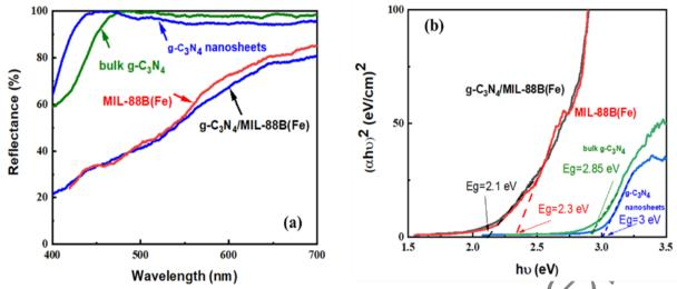
**Figure 4.** (a) DRS spectra and (b) Tauc's plots of bulk g-C<sub>3</sub>N<sub>4</sub>, g-C<sub>3</sub>N<sub>4</sub>, nanosheets, MIL-88B(Fe), and g-C<sub>3</sub>N<sub>4</sub>/MIL-88B(Fe) nanocomposite, calculated from DRS spectra and Tauc's equation. The extrapolation of the plots' linear ranges show the band gap energies (Eg).
