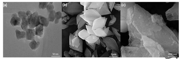
Figure 1. TEM image of (a) g-C3N4, SE micrographs of (b) pure MIL-88B(Fe) and (c) g-C3N4/MIL-88B(Fe) nanocomposite.
