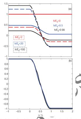
FIG.2: Color online: Spin current density of spin polarized carriers in the z direction ves location of the DW region normalized to the length of the DW region.  $k_FL=1$  and  $k_FL=10$  for panel (a) and (b).
