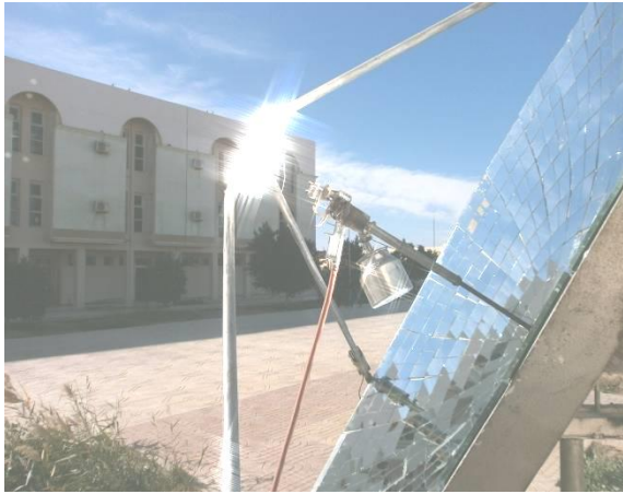
Figure 1 A photograph of the experimental setup for the deposition of F-doped NiO thin films.
