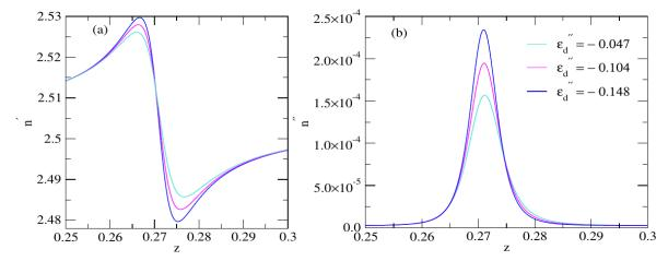
**Figure 6.** Active composite with dielectric coated metal spherical NCs with three different values of  $\varepsilon_d'' = 0.0$ ). n' versus z (a) and n'' versus z (b). Numerical values of composite parameters; metal fraction in the inclusion p = 0.7.
