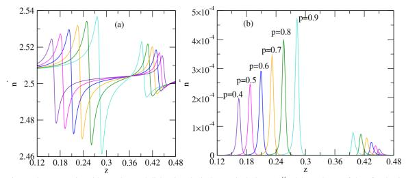
Figure 1. Passive composite with metal coated dielectric spherical Nano inclusions ( $\varepsilon_d$ '' = 0.0). Real part of the refractive index (n') versus the dimensionless frequency (z) (a) and imaginary part of the refractive index (n'') versus z (b). Numerical values of composite parameters; fraction of inclusions in the composite f = 0.001.
