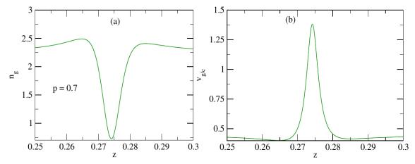
**Figure 11.** Passive composite with dielectric-metal spherical Nano inclusions ( $\varepsilon_d'' = -0.0$ ). Its group index  $n_g$  versus z (a). The normalized group velocity  $v_g/c$  versus z (b). Numerical values of composite parameters: metal fraction in an inclusion p = 0.7.
