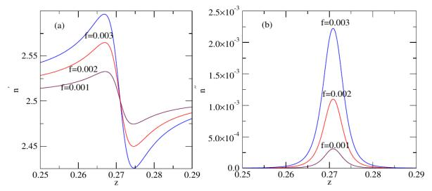
**Figure 5.** Active composite with dielectric coated metal spherical NCs ( $\varepsilon_d$ "=-0.20722). n' versus z (a) and n'' versus z (b). Numerical values of composite parameters; metal fraction in the inclusion p = 0.7.
