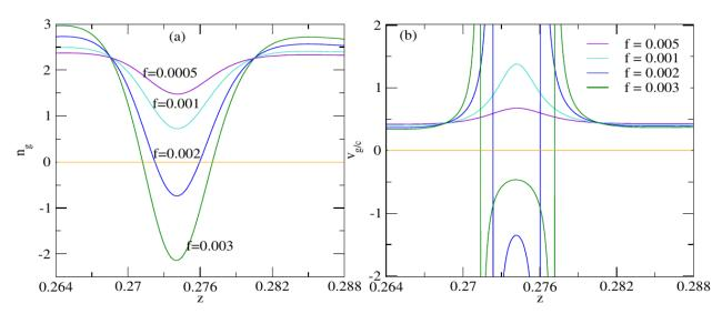
**Figure 13.** Passive composite with dielectric-metal spherical Nano inclusions ( $\varepsilon_d$ " = -0.0). Its group index  $n_g$  versus z (a). The normalized group velocity  $v_g/c$  versus z (b). Numerical values of composite parameters: metal fraction in an inclusion p = 0.7
