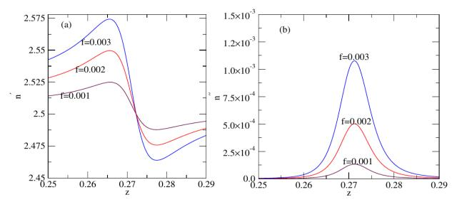
**Figure 4.** Passive composite with dielectric coated metal spherical NCs ( $\varepsilon_d''=0.0$ ). n' versus z(a) and n'' versus z(b). Numerical values of composite parameters; metal fraction in the inclusion p=0.7.
