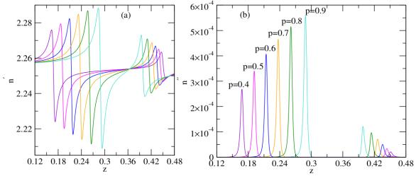
**Figure 2.** Active composite with metal coated dielectric spherical Nano inclusions ( $\varepsilon_d$ " = -0.20722). Real part of the refractive index (n') versus the dimensionless frequency (z) (a) and imaginary part of the refractive index (n'') versus z (b). Numerical values of composite parameters; fraction of inclusions in the composite f = 0.001.
