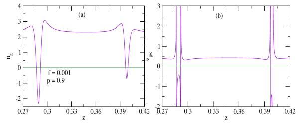
**Figure 8.** Active composite with metal-dielectric spherical Nano inclusions ( $\varepsilon_d'' = -0.20722$ ). Its group index  $n_g$  versus the dimensionless frequency z (a). The normalized group velocity  $v_g/c$  versus z (b). Numerical values of composite parameters: metal fraction in an inclusion p = 0.9, fraction of inclusions in the composite f = 0.00.1.
