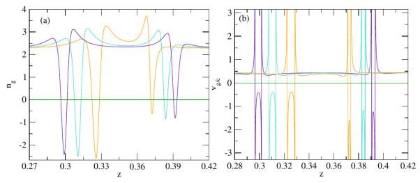
**Figure 10.** Active composite with metal-dielectric spherical Nano inclusions ( $\varepsilon_d'' = -0.20722$ ). Its group index  $n_g$  versus z (a). The normalized group velocity  $v_g/c$  versus z (b). Numerical values of composite parameters: three different metal fraction in an inclusion, fraction of inclusions in the composite f = 0.001.
