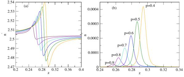
**Figure 3.** Passive composite with dielectric coated metal spherical NCs ( $\varepsilon_d$ "= 0.0). n'versus z (a) and n"versus z (b). Numerical values. of composite parameters; metal fraction in the inclusion p = 0.4, 0.6, 0.7, 0.8,and 0.9, fraction of inclusions in the composite f = 0.001.
