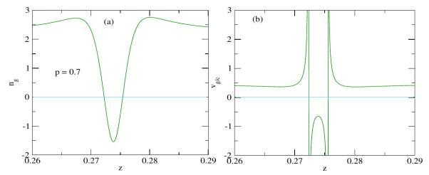
**Figure 12.** Active composite with dielectric-metal spherical Nano inclusions ( $\varepsilon_a'' = -0.20722$ ). Its group index  $n_g$  versus z (a). The normalized group velocity  $v_g/c$  versus z (b). Numerical values of composite parameters: metal fraction in an inclusion p = 0.7.
