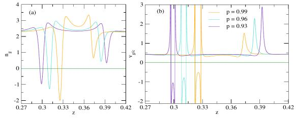
Figure 9. Passive composite with metal-dielectric spherical Nano inclusions ( $\varepsilon_d'' = -0.0$ ). Its group index  $n_g$  versus z (a). The normalized group velocity  $v_g/c$  versus z (b). Numerical values of composite parameters: three different metal fraction in an inclusion, fraction of inclusions in the composite f = 0.001.
