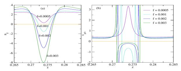
**Figure 14.** Active composite with dielectric-metal spherical Nano inclusions ( $\varepsilon_d'' = -0.20722$ ). Its group index  $n_g$  versus z (a). The normalized group velocity  $v_g/c$  versus z (b). Numerical values of composite parameters: metal fraction in an inclusion p = 0.7.
