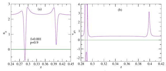
**Figure 7.** Passive composite with metal-dielectric spherical Nano inclusions ( $\varepsilon_d''=0$ ). Its group index  $n_g$  versus the dimensionless frequency z (a). The normalized group velocity  $v_g/c$  versus z (b). Numerical values of composite parameters: metal fraction in an inclusion p = 0.9, fraction of inclusions in the composite f = 0.001.
