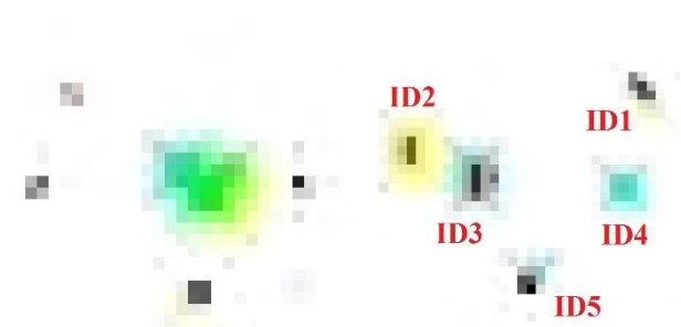
Fig. 4. A cut of a negative RAW image file took by the 12.3-megapixel camera. (Left) Some spots with different sizes and values. (Right) Two connected spots (ID2, ID3) distinguished by the analysis.
