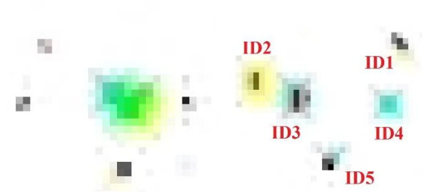
Figure 4. A cut of a negative RAW image file took by the 12.3-megapixel camera. (Left) Some spots with different sizes and values. (Right) Two connected spots (ID2, ID3) distinguished by the analysis.
