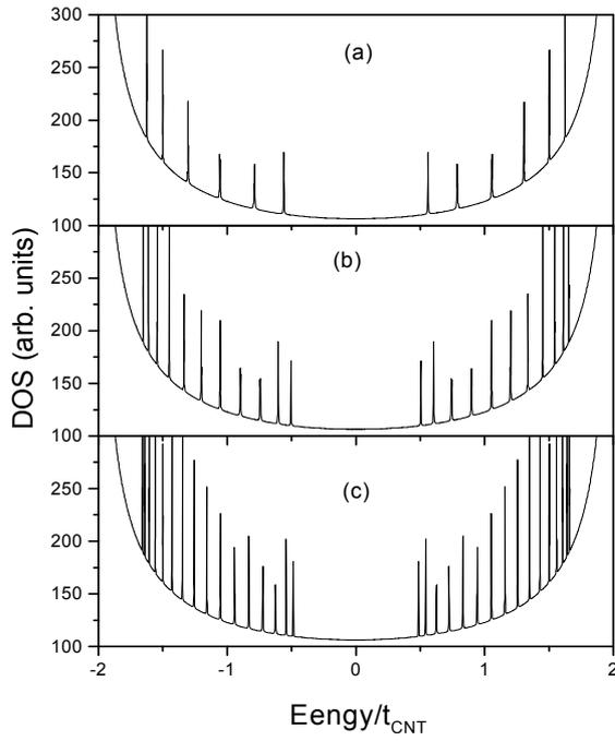
**Figure 2.** A plot of the electronic DOS vs the dimensionless parameter  $\text{Energy}/t_{\text{CNT}}$  for the CNT/*trans*-PA/CNT system with the parameters of  $t_{\text{CNT}}=3\text{ eV}$  and  $t_c=0.3\text{ eV}$  as described in the text. Plots (a)-(c) show the results for the molecules with 11, 21 and 31 atoms, respectively.
