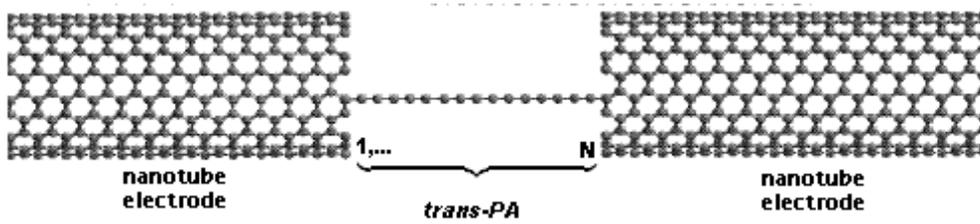
**Figure 1.** A schematic representation of the CNT/*trans*-PA/CNT structure as described in the text.
