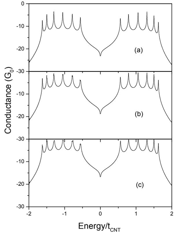
**Figure 5.** Conductance in units of  $G_0$  vs the dimensionless parameter  $\text{Energy}/t_{CNT}$  for the CNT/*trans*-PA/CNT system with  $t_{CNT} = 3$  eV. Plots (a)-(c) show the results for the molecule with 11 atoms and  $t_c = 0.1, 0.2$  and  $0.3$  eV, respectively.
