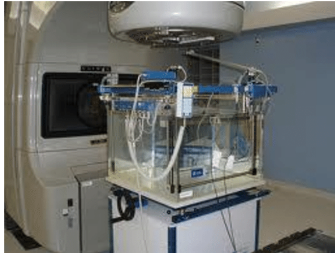
Figure 3. Experimental set-up for measuring TPR_{20,10} .
