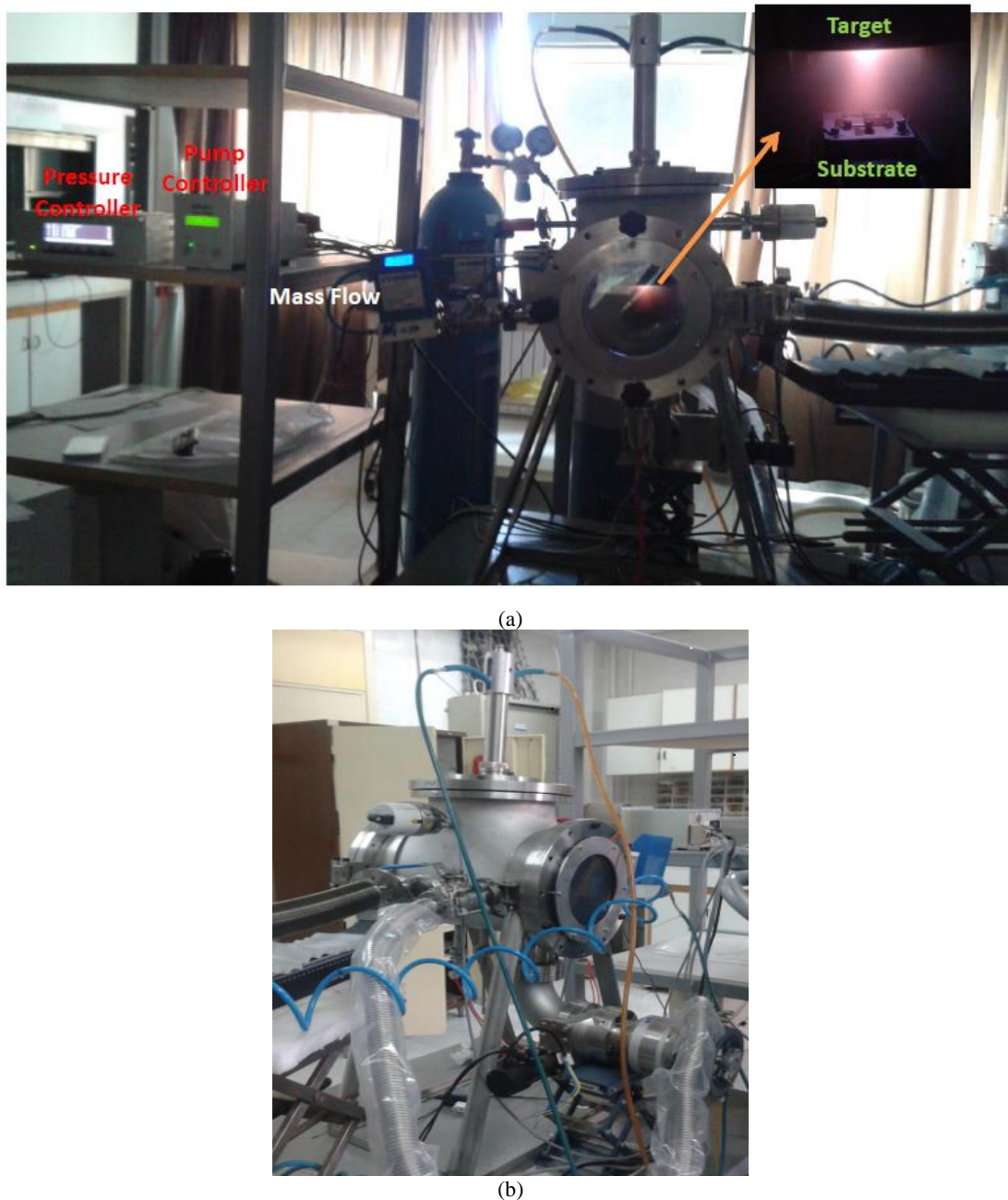
Figure 1. Experimental set-up of DC magnetron sputtering, (a) with plasma and (b) without plasma.
