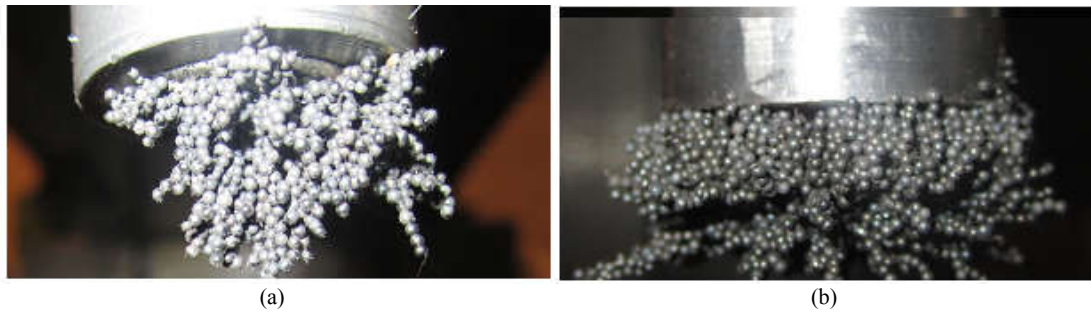
Figure 25. (color onlin) (a) Non-ferromagnetic magnet fixture, and (b) ferromagnetic magnet fixture.
