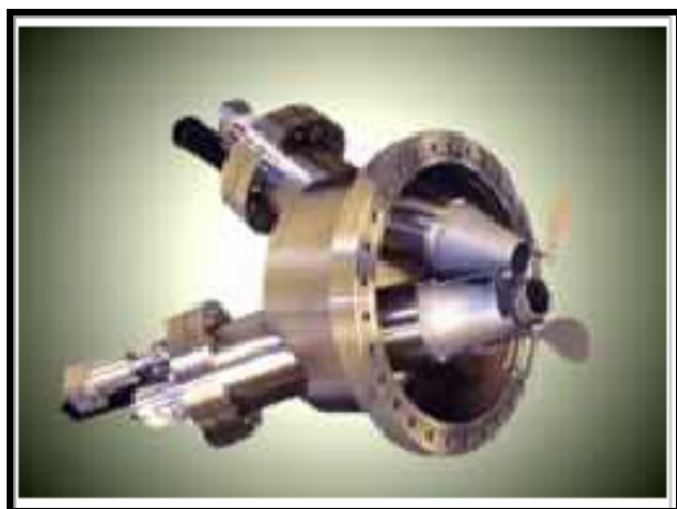
Figure 8. (color online) Cluster flange arrangement for 3 sputtering guns.
