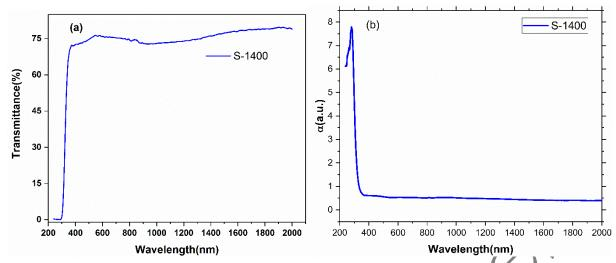
Fig. 3. (a) Transmission spectra and (b) absorption coefficient vs wavelength for (S-1400+ethylen glycol on glass
