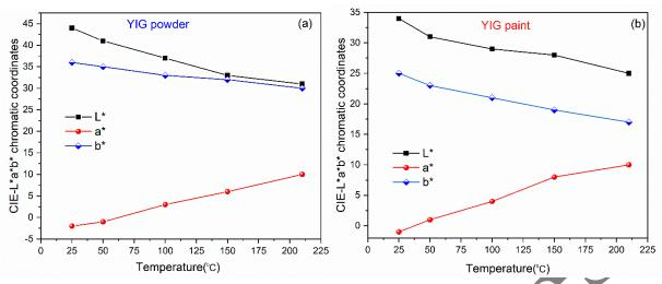
Fig. 6. Variation of Chromatic coordinates of (a) YIG powder and (b) YIG paint versus temperature.
