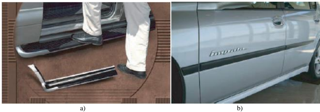
Figure 10. TPO nanocomposites: application for automotive parts [139]: (a) M-Van step Assist: first commercial launch and (b) impala: second nanocomposite application. Through the courtesy of M. Verbrugge, General Motors.
